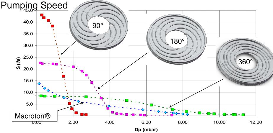
•Pumping speed up to 45 l/s is possible with an "open" 90° spiral design
