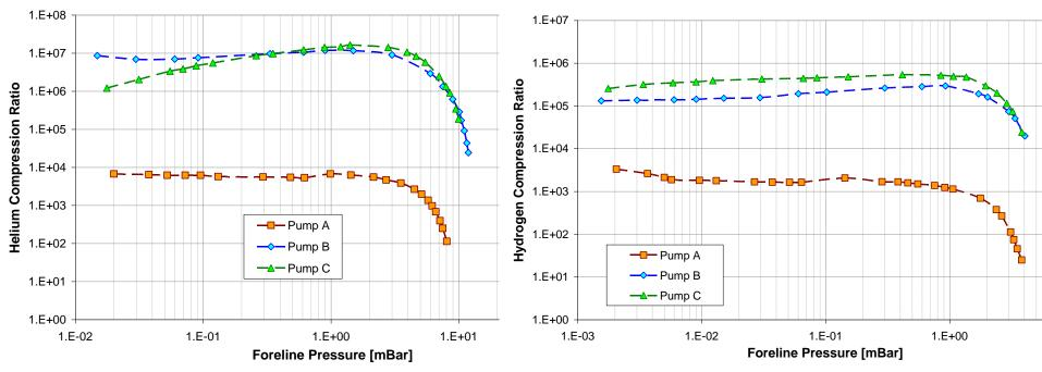
•TMDP equipped with TwisTorr stages largely outperform MacroTorr TMDP
